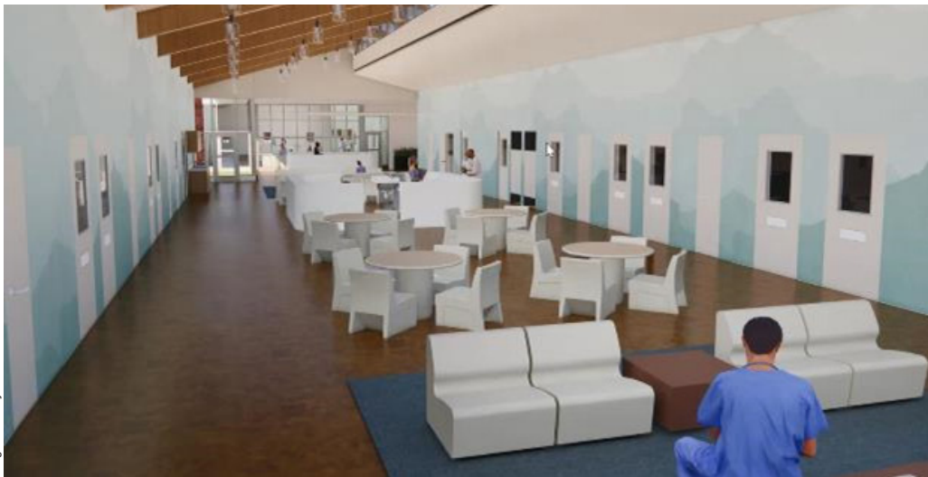
In support of biophilia and WELL, this dayroom in the mental health treatment building features natural light via clerestory windows, wall graphics of nature, acoustical panels and exposed wood beams.
